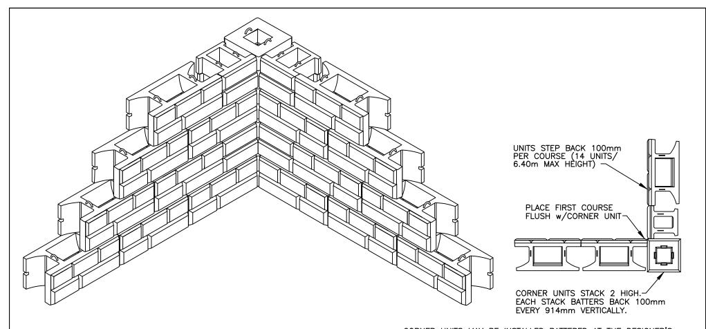
CORNER UNITS MAY BE INSTALLED BATTERED AT THE DESIGNER'S DISCRETION. ADJACENT COURSES MAY NEED TO BE TRIMMED OR INSTALLED OFF RUNNING BOND DEPENDING ON END WALL CONDITIONS.
