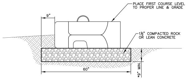
NOTE: BEARING CONDITIONS SHALL BE OBSERVED BY THE SITE GEOTECHNICAL ENGINEER. BASE DIMENSIONS MAY BE INCREASED TO ADDRESS DEFICIENT SOIL BEARING CONDITIONS.
