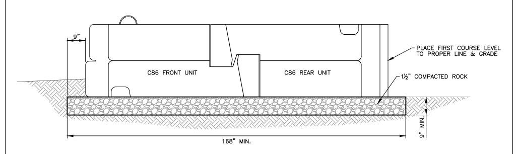
NOTE: BEARING CONDITIONS SHALL BE OBSERVED BY THE SITE GEOTECHNICAL ENGINEER. BASE DIMENSIONS MAY BE INCREASED TO ADDRESS DEFICIENT SOIL BEARING CONDITIONS.
