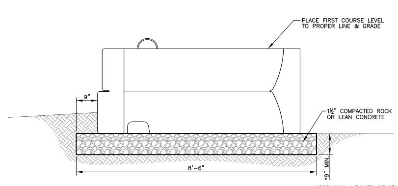
NOTE: BEARING CONDITIONS SHALL BE OBSERVED BY THE SITE GEOTECHNICAL ENGINEER. BASE DIMENSIONS MAY BE INCREASED TO ADDRESS DEFICIENT SOIL BEARING CONDITIONS.
