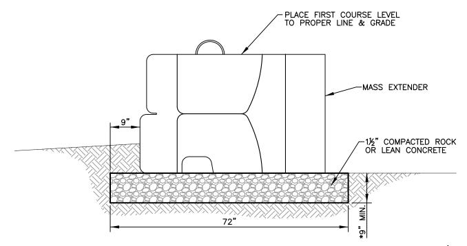
NOTE: BEARING CONDITIONS SHALL BE OBSERVED BY THE SITE GEOTECHNICAL ENGINEER. BASE DIMENSIONS MAY BE INCREASED TO ADDRESS DEFICIENT SOIL BEARING CONDITIONS.
