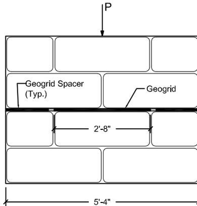
$$\text{Normal Force } \left( \frac{\text{kips}}{\text{ft}} \right) = \frac{P \text{ kips}}{8 \text{ ft}}$$
