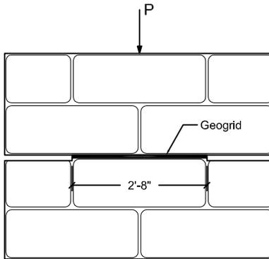
$$\text{Normal Force } \left( \frac{\text{kips}}{\text{ft}} \right) = \frac{P \text{ kips}}{4 \text{ ft}}$$
