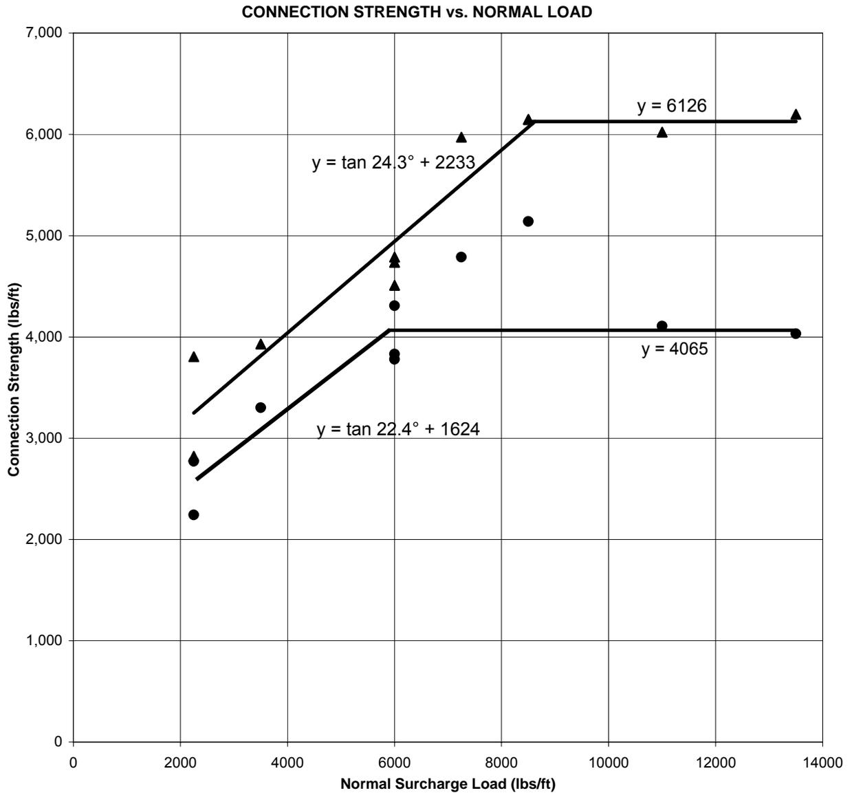
**INTERFACE SHEAR TESTS**
